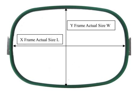
"X direction frame size" and "Y direction frame size" should be set according to the actual size of different frames. Note: this parameter need be set according to the actual embroidery range of the frame, for the apparel frame is usually not square.
